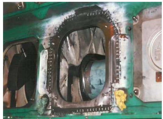
Removing The Damaged Engine Door And Metal Stitching In A New Insert.
